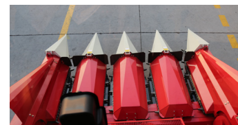
Matched header for wheat 2.56m/2.57m, 4/5 rows header for corn
