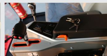
Suspension operating table, height-adjustable, one-bar control
