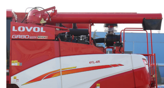
4.5m Raise and lower adjustable, bigger(φ650px) unloading pipe+low-auger, unloading time is 53s from full grain tank
