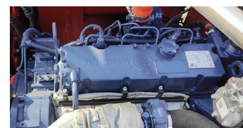
Weichai Engine 190hp, 63cc hydraulic pump+63cc hydraulic motor, travelling speed 40km/h.
