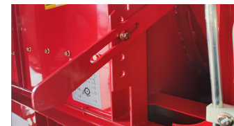
The gap of concave can be adjusted 6 levels, which has good effect for different working conditions and crops
