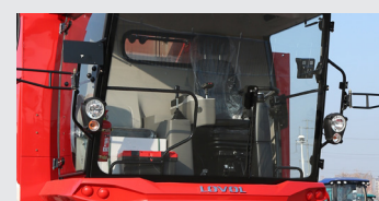
2.1 m wide sealed positive pressure cab, equipped with passenger seat
